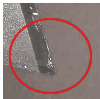
Endurance for long distances: The edge rounding of a diamond saw tooth after 80 km of cutting.
