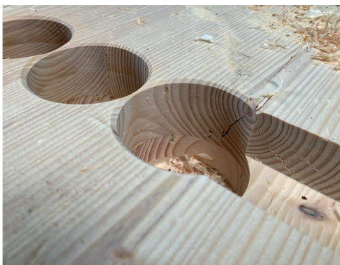
Holes made by LEUCO: clear test result for the t3-System cutter – excellent milling quality, excellent edge quality, no burn marks. The chamfer with 45 degrees at the upper edge is produced by the innovative tool in one pass.
