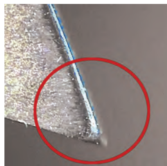
Very effective over short distances: The edge rounding of a carbide saw tooth after 4 km of cutting.
