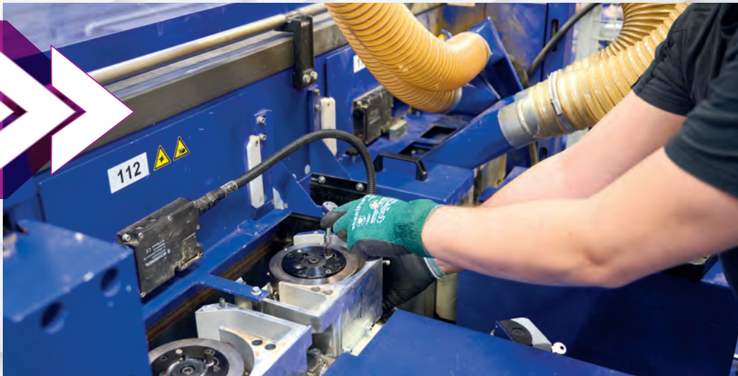
Efficiency under control at the kitchen manufacturer Ballerina: The employees “resharpen” the cutting edges on the LEUCO milling cutter by small turn with an Allen key - minimum machine downtime, maximum tool utilization, flawless product quality.
